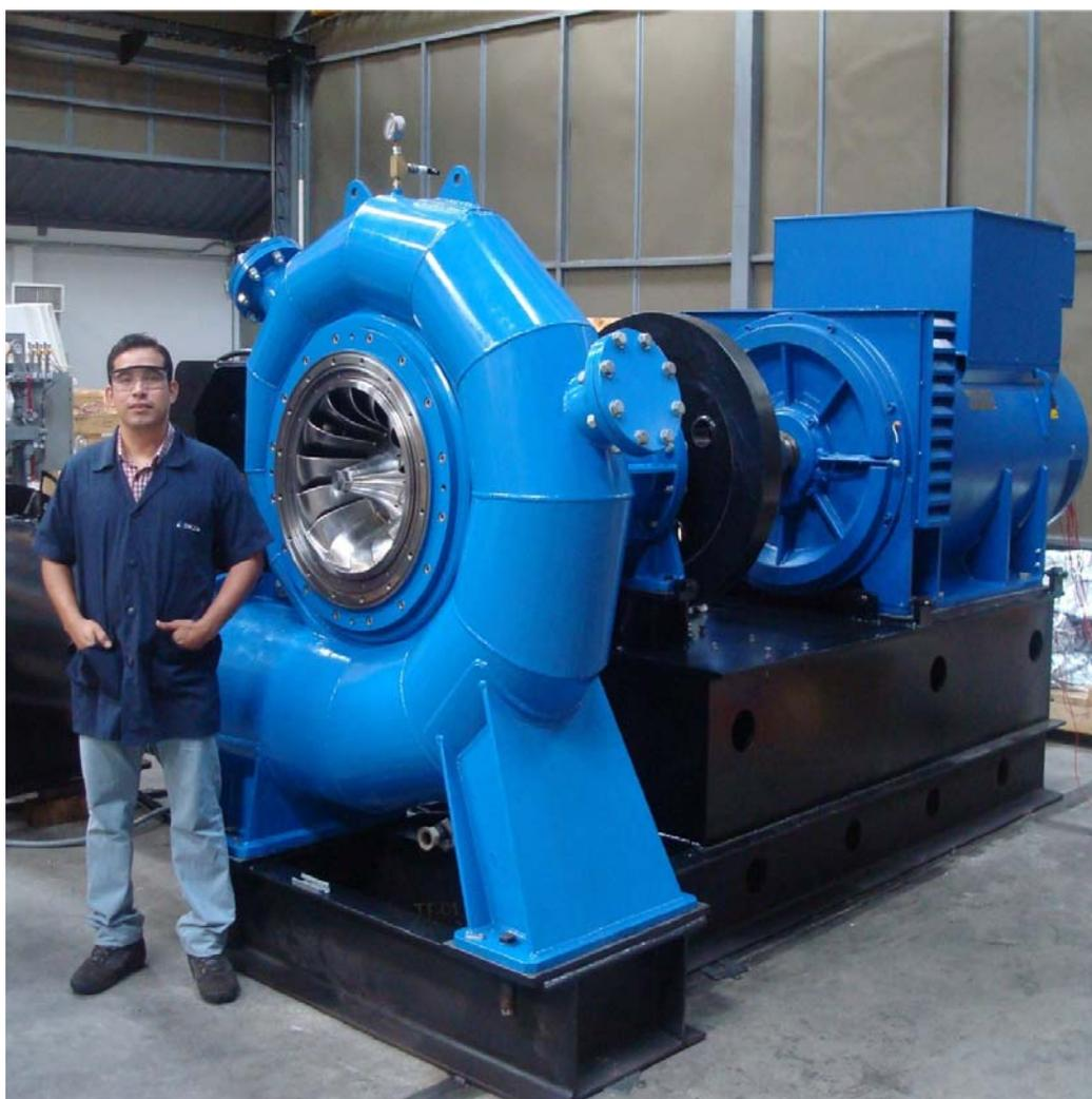
FIGURA 2.16 TURBINA FRANCIS PROYECTO HIDROMIRA, 1MW.
