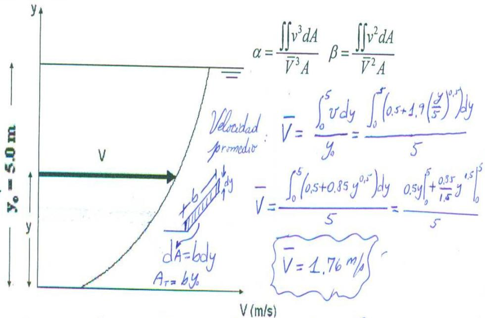
$$\beta: \beta = \frac{\iint v^2 dA}{\bar{V}^2 A} = \frac{b \int_0^5 v^2 dy}{\bar{V}^2 [b y_0]} = \frac{\int_0^5 v^2 dy}{(\bar{V})^2 (5)} = \frac{\int_0^5 (0.5 + 0.85 y^{0.5})^2 dy}{(1.76)^2 (5)} = \frac{\int_0^5 (0.5)^2 + 2(0.5)(0.85) y^{0.5} + 0.85^2 y dy}{15.6}$$
