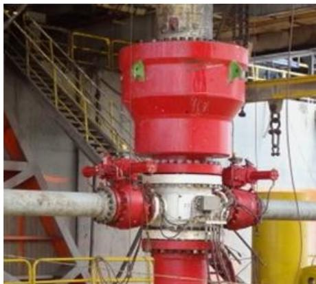
Figura 1.31 Diverter (FUENTE: JVS Engineers, [www.jvsengg.com/pressure-diverter-ball-valve.html](http://www.jvsengg.com/pressure-diverter-ball-valve.html))
