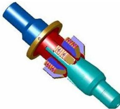
Figura 4.10 Die Collar (FUENTE: <http://www.ingenieriadepetroleo.com/2010/11/herramientas-empleadas-en-la-pesca-de.html>)
