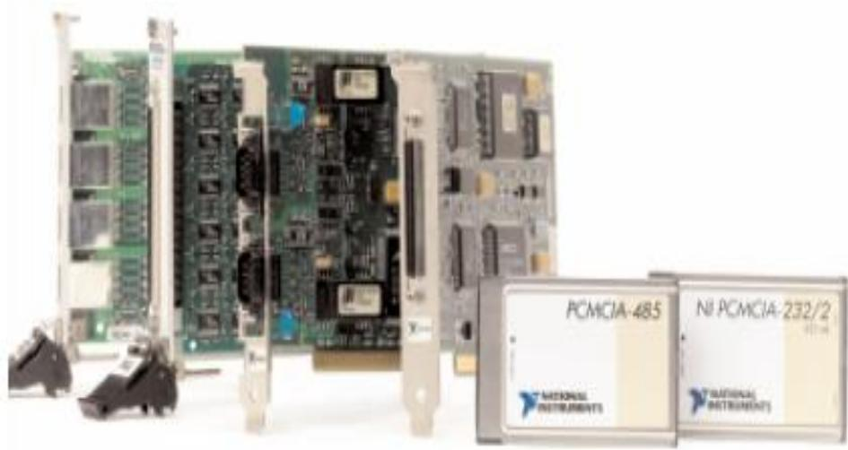
**Figura 4. 3 NI PXI-8431/8: INTERFACES SERIALES PARA PXI, PCI, PCMCIA, ETHERNET, Y USB. [15]**
