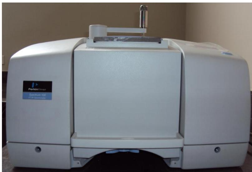
**FIGURA 3.20 ESPECTRÓMETRO PERKIN ELMER SPECTRUM 100**
