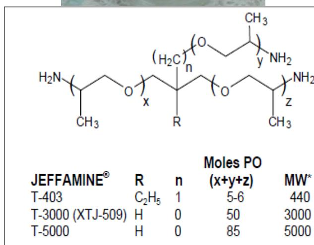
**FIGURA 2.9. AMINA LÍQUIDA Y ESTRUCTURA
