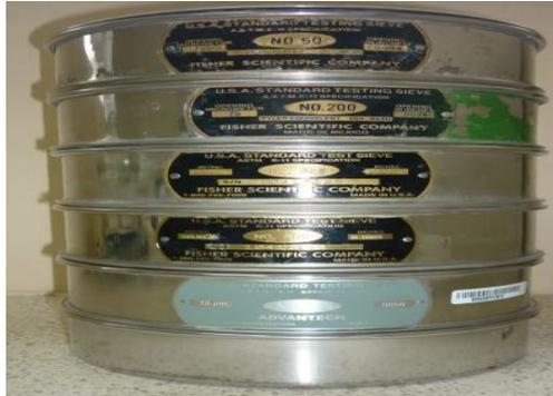
**FIGURA 3.15. MALLAS ASTM USADAS EN EL PROYECTO**
