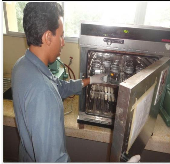
**FIGURA 3.55. PUESTA AL HORNO DE LA MEZCLA RESINA
