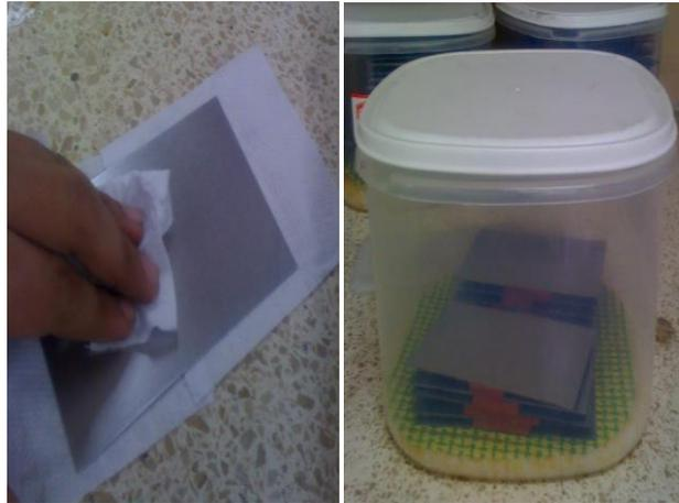
**FIGURA 3.83 LIMPIEZA Y ALMACENAMIENTO DE PLACAS RECTANGULARES**
