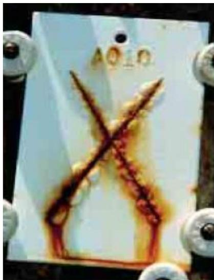
**FIGURA 2.2. PROBETA METÁLICA EVALUADA CON RECUBRIMIENTO ANTICORROSIVO MEDIANTE NORMAS. [9]**
