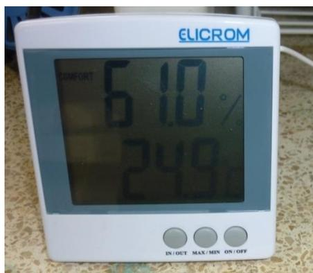
**FIGURA 2.15. HIGRÓMETRO DIGITAL**
