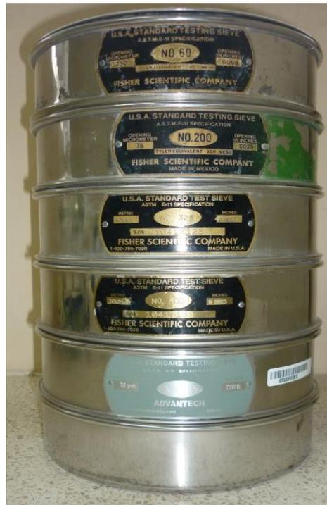
**FIGURA 2.25. MALLAS ASTM**
