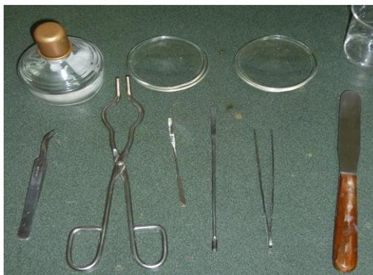
**FIGURA 2.19. MECHERO – VIDRIO RELOJ –PINZAS-
