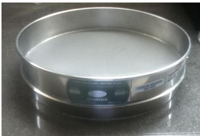
**FIGURA 2.8. MALLA ASTM #270**
