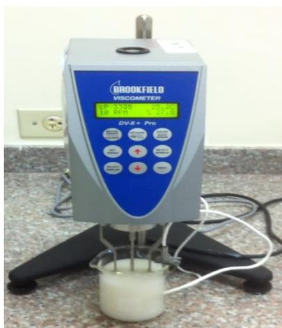
**FIGURA 3.4 VISCOSÍMETRO BROOKFIELD (DV-II +PRO)**
