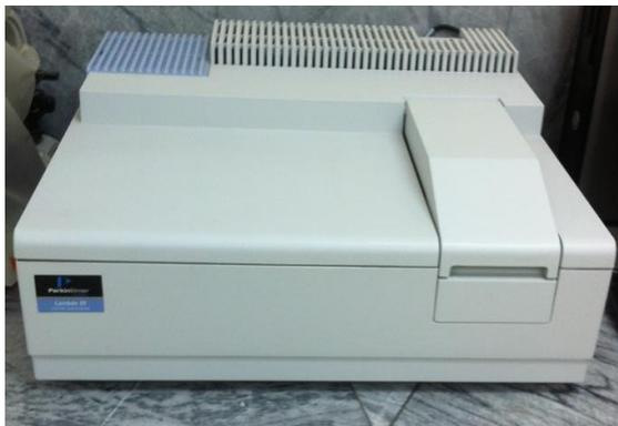
**FIGURA 3.3 ESPECTROFOTÓMETRO UV/VIS PERKINELMER
