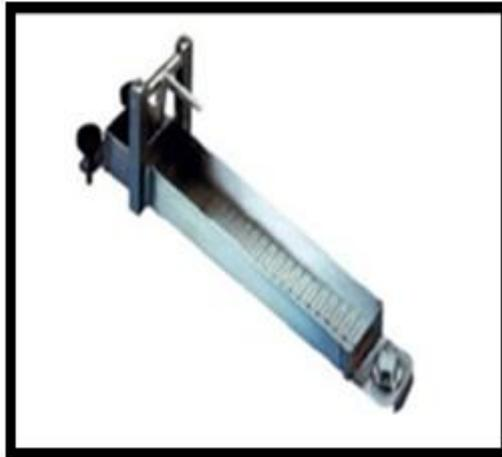
**FIGURA 2.1 CONSISTÓMETRO BOSTWICK [3]**
