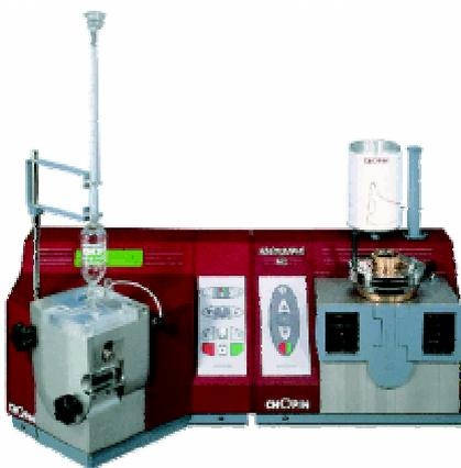
**FIGURA 2.1. ALVEOCONSISTÓGRAFO**
