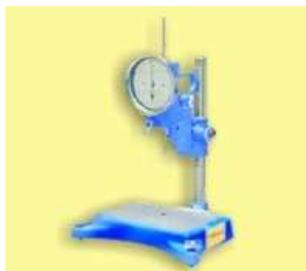
**FIGURA 2.2. PENETRÓMETRO**
