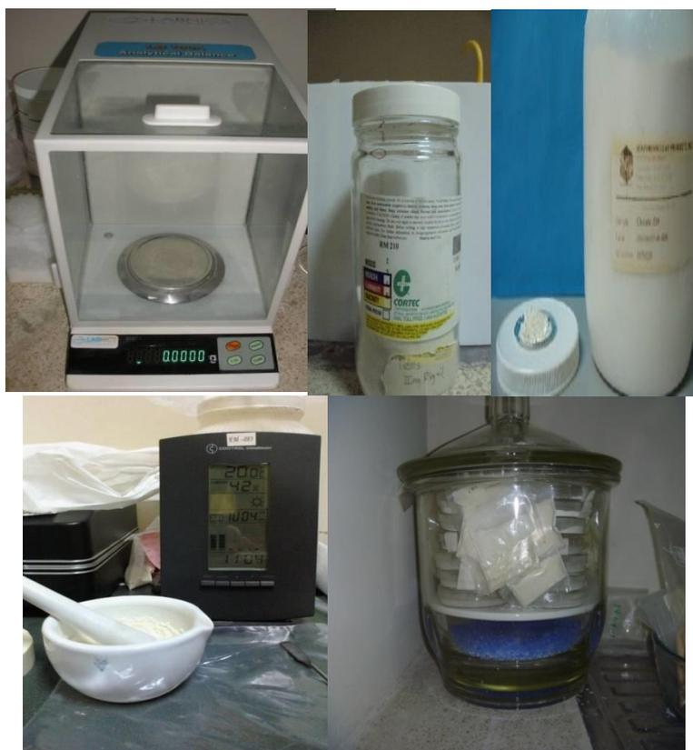
**FIGURA 3.16 PROCEDIMIENTO DEL MÉTODO SECO.**
