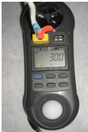
**FIGURA 3.14. ANEMÓMETRO Y TERMOCUPLA TIPO K.**
