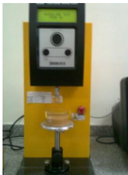
FIGURA 3.11 CT3- Texture Analyzer.
