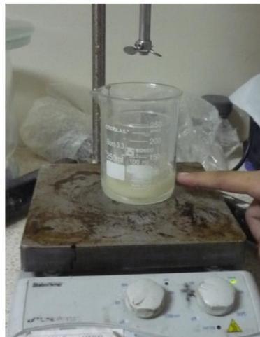
**FIGURA 3.38 COLOCAR VASO CON LA MEZCLA EPÓXICO-
