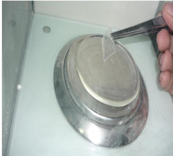
**FIGURA 3.52 PESAR LA MUESTRA EN LA BALANZA**
