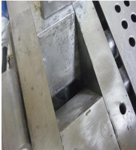
**FIGURA 3.26 RANURA PARA COLOCAR LA MEZCLA**
