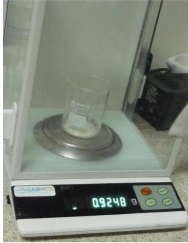
**FIGURA 3.22 PESAR LA MEZCLA ARCILLA-INHIBIDOR**
