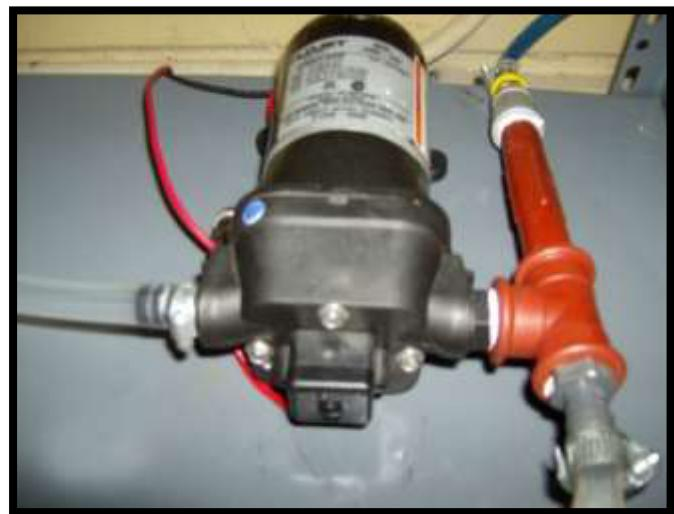
**Figura 1.7 – Bomba FLOJET 12 VDC**
