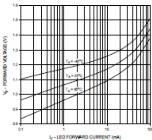
Figure 2. On-State Characteristics
