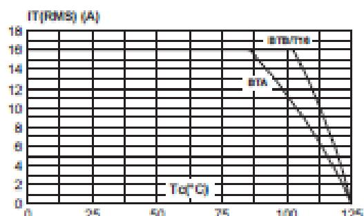
Fig. 2-2: DPAK RMS on-state current versus ambient temperature (printed circuit board FR4, copper thickness: 35 µm), full cycle.
