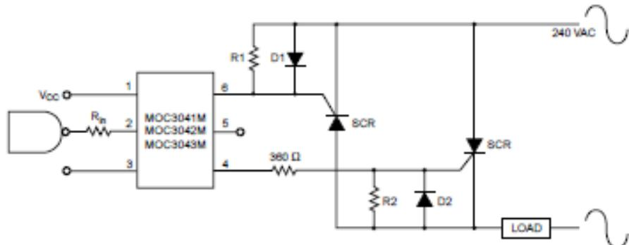
Figure 16. Inverse-Parallel SCR Driver Circuit
