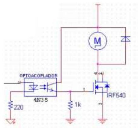
**Figura 2.4 – Diagrama circuito control bomba**
