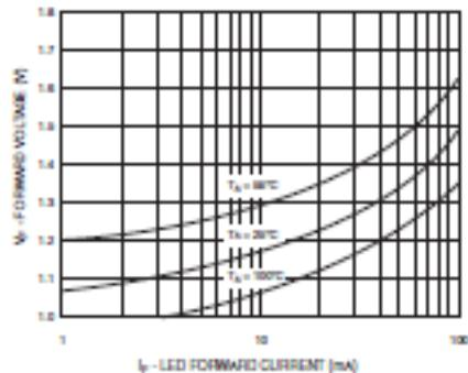
Fig. 2 LED Forward Voltage vs. Forward Current
