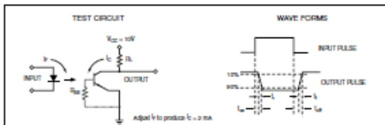
Figure 20. Switching Time Test Circuit and Waveforms
