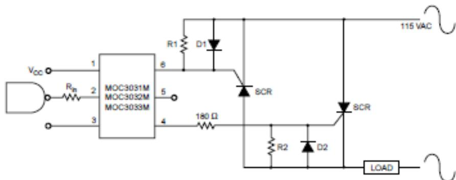
Figure 14. Inverse-Parallel SCR Driver Circuit
