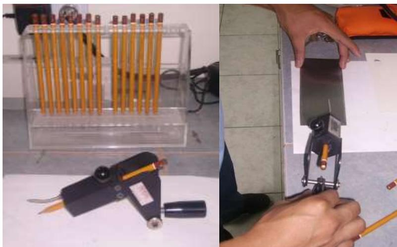
**FIGURA 3.31. PRUEBA DE DUREZA AL LÁPIZ INEN 1001.**
