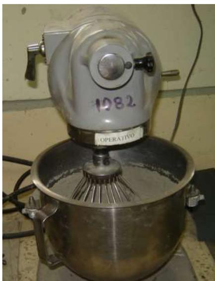
**FIGURA 3.10 HOMOGENEIZADO DE LA MEZCLA CEMENTO-ZEOLITA EN SECO**
