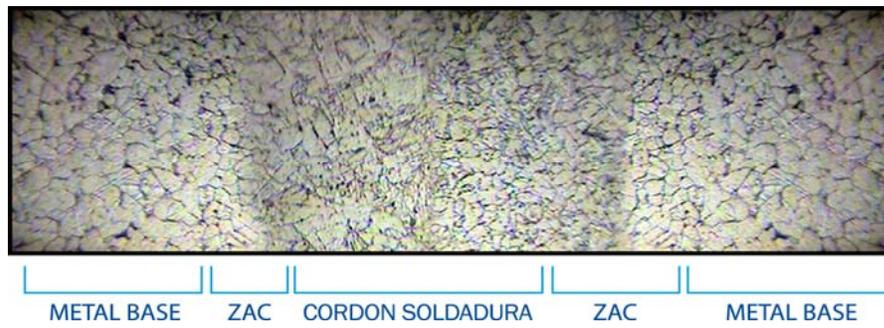
**FIGURA 2.7. MICROESTRUCTURA PROVEEDOR CST. 1.9 MM
