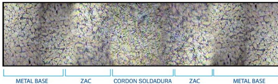
**FIGURA 2.8. MICROESTRUCTURA PROVEEDOR CST. 1.5 MM
