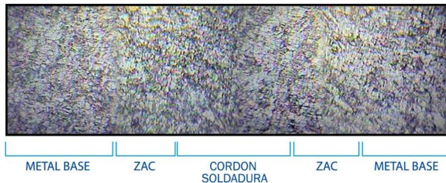
**FIGURA 2.10. MICROESTRUCTURA PROVEEDOR USIMINAS 0.9 MM
