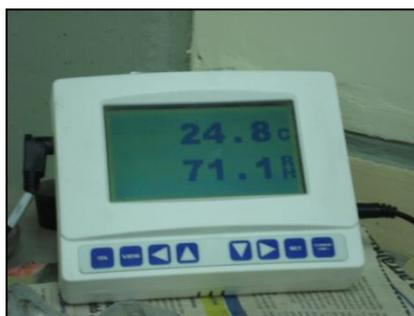
**FIGURA 3.14** MEDIDOR DIGITAL DE TEMPERATURA Y HUMEDAD RELATIVA.
