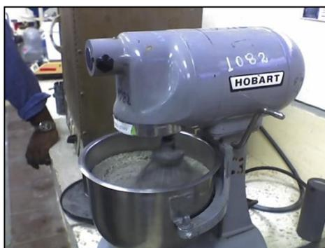
**FIGURA 3.15** MEZCLA HOMOGÉNEA CEMENTO-ZEOLITA EN SECO
