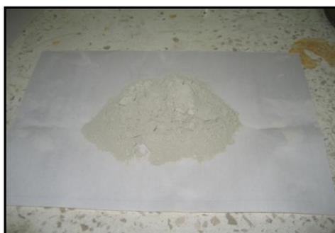
**FIGURA 3.10** ZEOLITA CON GRANULOMETRÍA FINAL 45  $\mu\text{m}$
