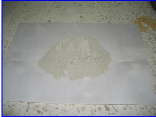
**FIGURA [3.17] ZEOLITA CON GRANULOMETRÍA FINAL 45  $\mu\text{m}$**
