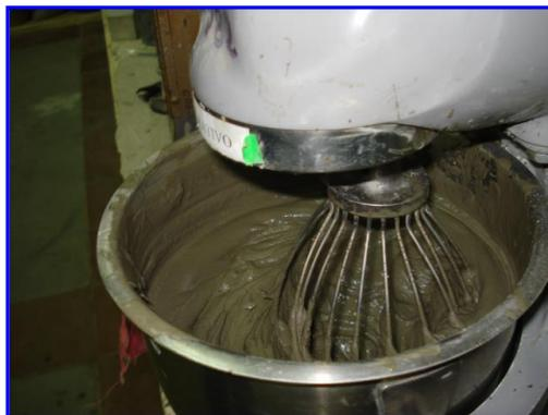
**FIGURA [3.22] CEMENTO + ZEOLITA + AGUA EN LA MEZCLADORA**
