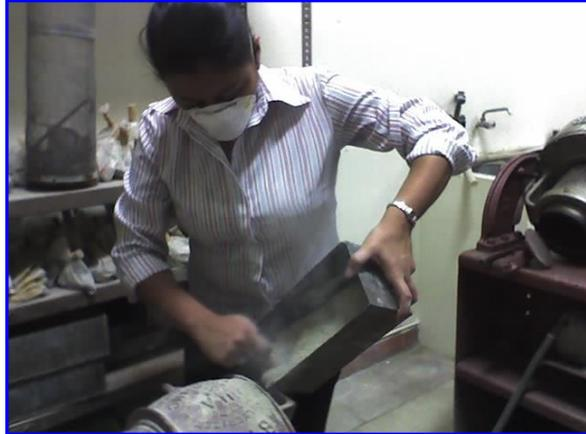
**FIGURA [3.11] AGREGANDO MATERIAL AL MOLINO DE DISCOS**
