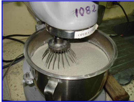
**FIGURA [3.21] HOMOGENEIZANDO CEMENTO + ZEOLITA EN SECO**
