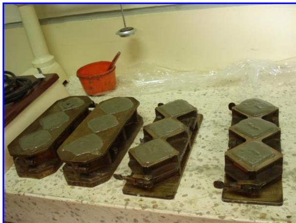
**FIGURA [3.25] PROBETAS REPOSANDO POR UNOS
