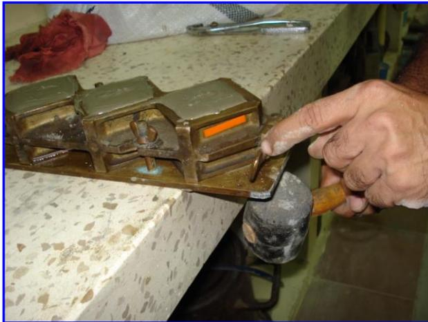
**FIGURA [3.24] COMPACTANDO LAS PROBETAS**
