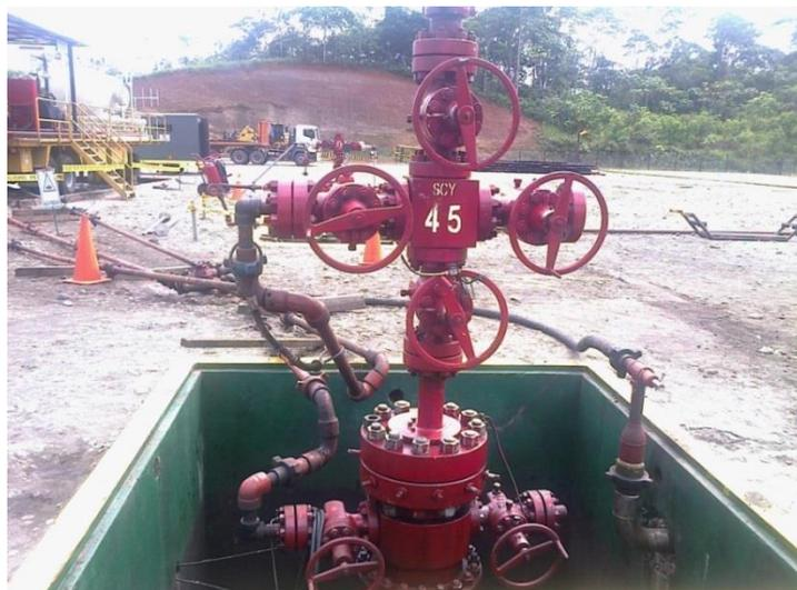
**FIGURA 2.14: Cabezal**
