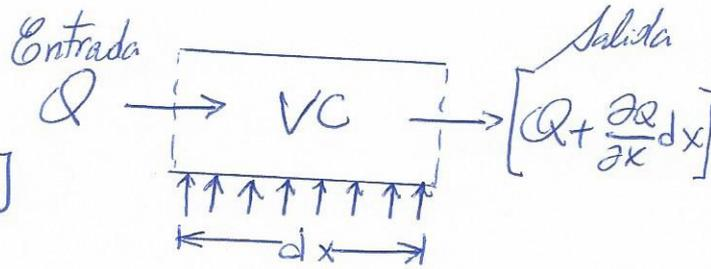
a)  $\left\{ \frac{\partial A}{\partial t} + \frac{\partial Q}{\partial x} - q = \phi \right\}$  Ecuación General 5/5
