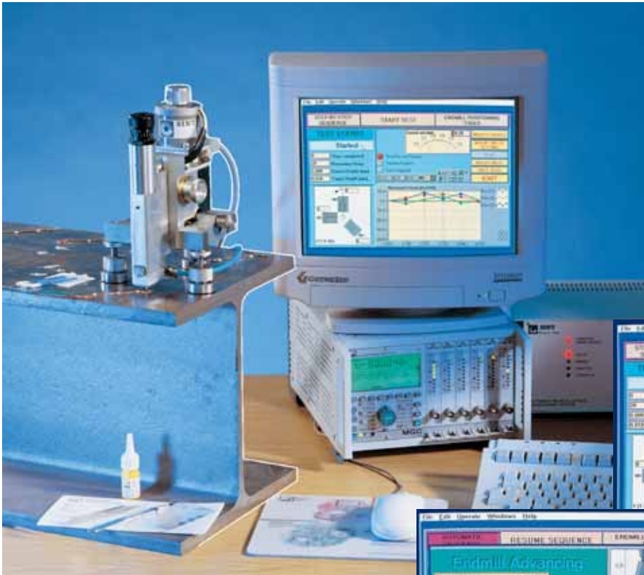
Complete measuring chain with amplifier and control and analysis PC
