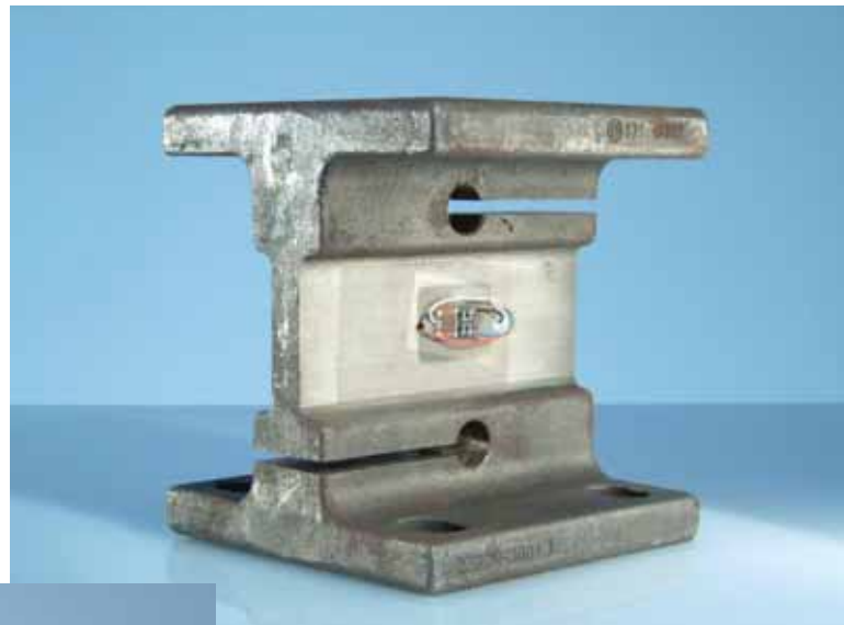
Strain gage installation on a customized machine element
