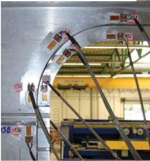
Strain gages in railway engineering
