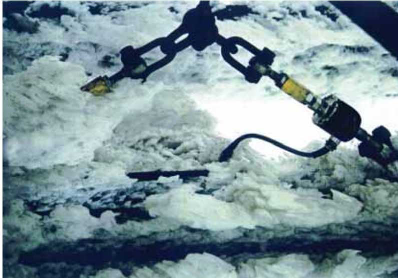
Tensile force measurement using C series strain gages at low temperatures (permafrost)
