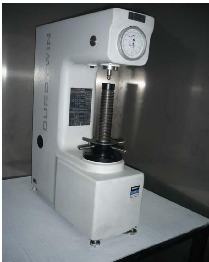
FIGURA 2.27 DURÓMETRO
