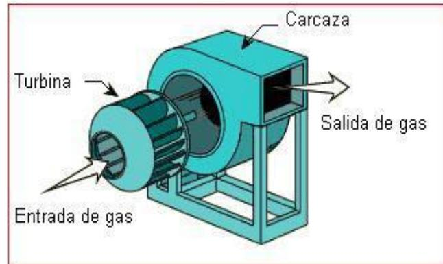
**FIGURA 2.19 VENTILADOR CENTRÍFUGO**
