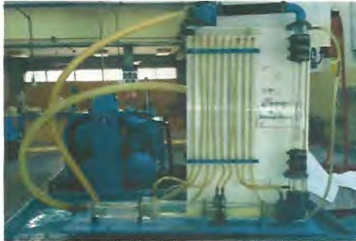
**FIGURA 4 TECQUIPMENT H10 (BANCO MEDIDOR DE FLUJO)**
