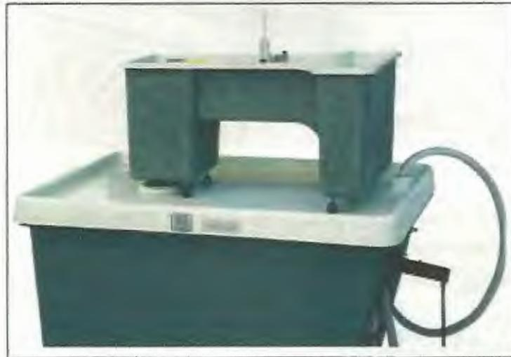
**FIGURA 3. BANCO HIDRÁULICO GRAVIMÉTRICO (TECQUIPMENT H1) SUMINISTRANDO FLUJO A UN EQUIPO EXPERIMENTAL<sup>1</sup>.**
