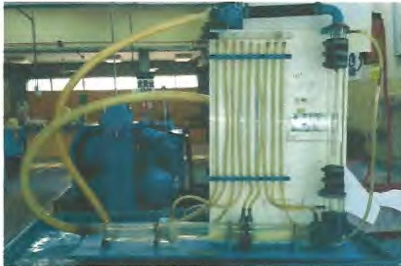
**FIGURA 4.3 TECQUIPMENT H10 (BANCO MEDIDOR DE FLUJO)**
