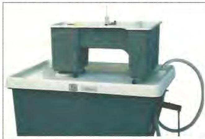
**FIGURA 4.1 BANCO HIDRÁULICO GRAVIMÉTRICO (TECQUIPMENT H1) SUMINISTRANDO FLUJO A UN EQUIPO EXPERIMENTAL<sup>15</sup>.**
