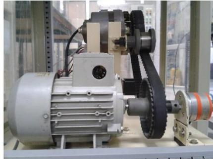
Figura 4.4 Acople motor-encoder
