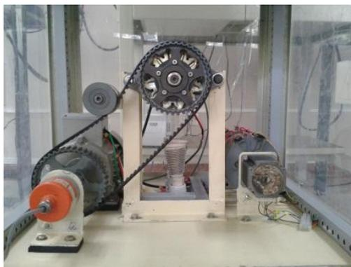
Figura 4.3 Acople motor-alternador
