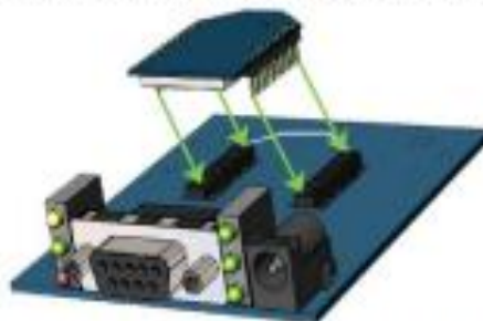
Figure 1-82. Xbee Series 2 Module Mounting to an RS-232 Interface Board.
