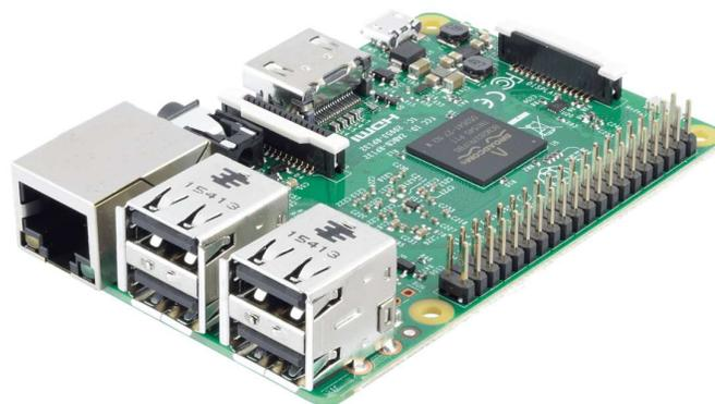
Figura 2.4: Raspberry pi 3 modelo B [14]
