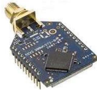
**Figura 2.8: Módulo XBEE PRO RPSMA Conector [21].**
