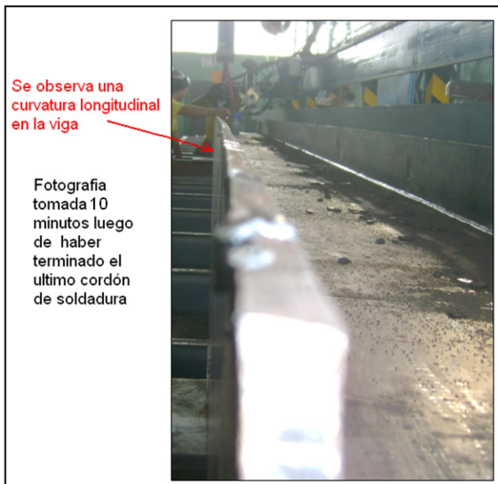
**FIGURA 4.44: CURVATURA EN LA VIGA I**
