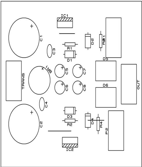
Fig. 6: Layout componentes
