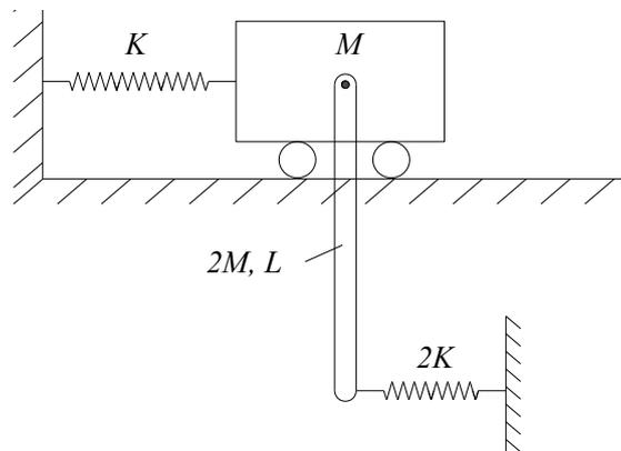
2.- You have to analyze the torsional vibration of a simplified shafting system of a fishing vessel (440 hp @1800 rpm, 6 cylinders, 4 stroke cycle, gear ratio of 2.5:1,  $Z_{prop}$ : 4). Employing Holzer method, estimate the second torsional natural frequency different from zero. (25):
