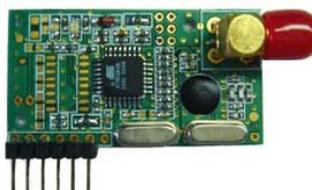
Figura 3.15 – Módulo RF HM-TR/TTL [13]
