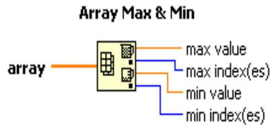
Returns the maximum and minimum values found in **array**, along with the indexes for each value.
