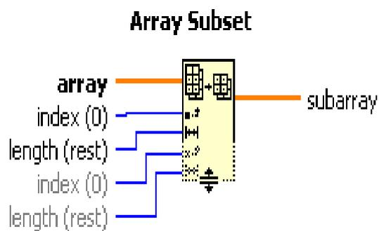
Returns a portion of **array** starting at **index** and containing **length** elements.
