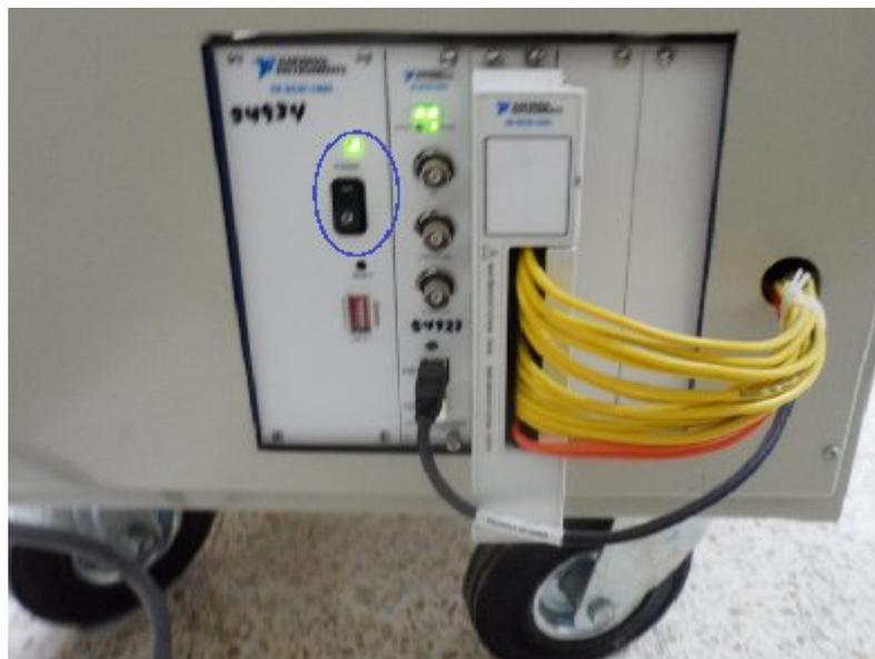
Figura A - 18 Chassis NI-SCXI 1000
