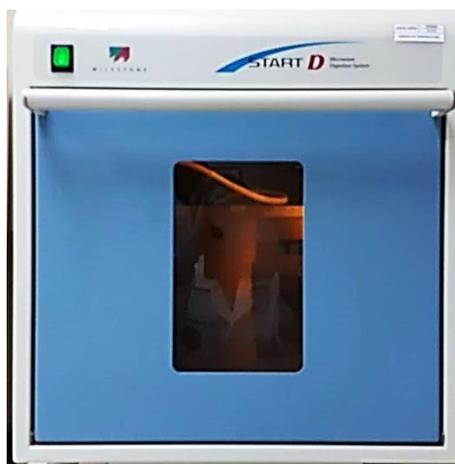
**Figura 37: Start Microwave Digestion System**
