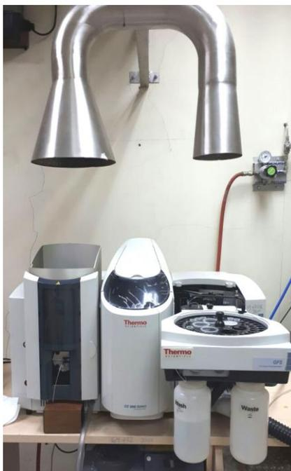
**Figura 38: Thermo Scientific ICE 3000 SERIES AA Spectrometer**
