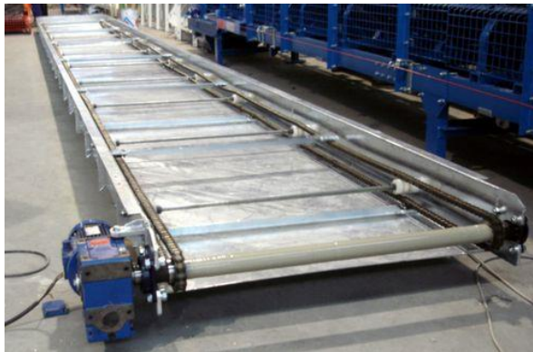
Figura 2.3 Transportador redler (Fuente: Tomado de https://www.cintasa.com/en/products/other-products/redler-conveyors/ )
