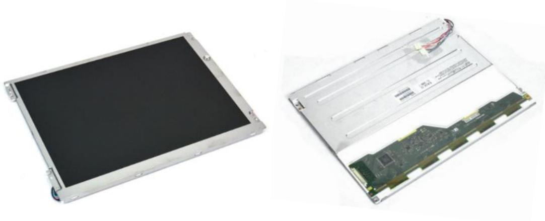
**Figura 4.53 Pantalla LCD TFT 12.1” Sharp. [92]**
