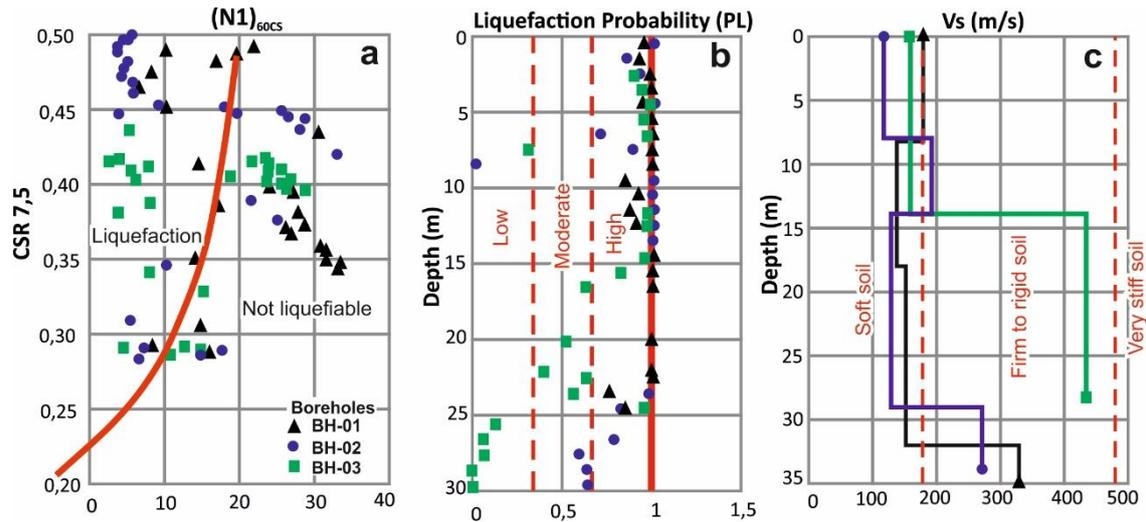
**Figure 5.** a) Relationship between the Cyclic Stress Ratio (CSR) causing liquefaction and the value  $(N1)_{60cs}$  for silty sands. b) Calculations obtained of liquefaction probability PL for sands from geoenvironmental drilling for the city of Jama. c) Evaluation of S-velocity ( $V_s$ ) to a depth of 35 m.
