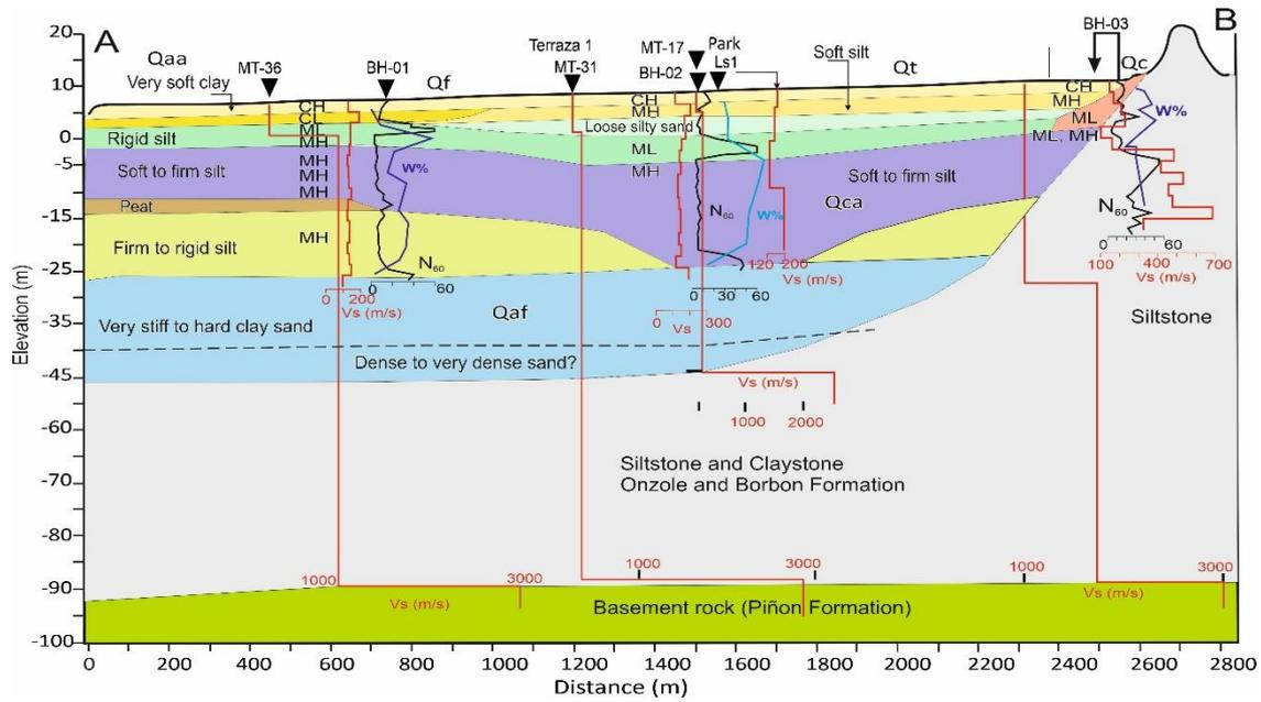
**Figure 4.** Geological - geoseismic section A-B of the urban area of Jama.
