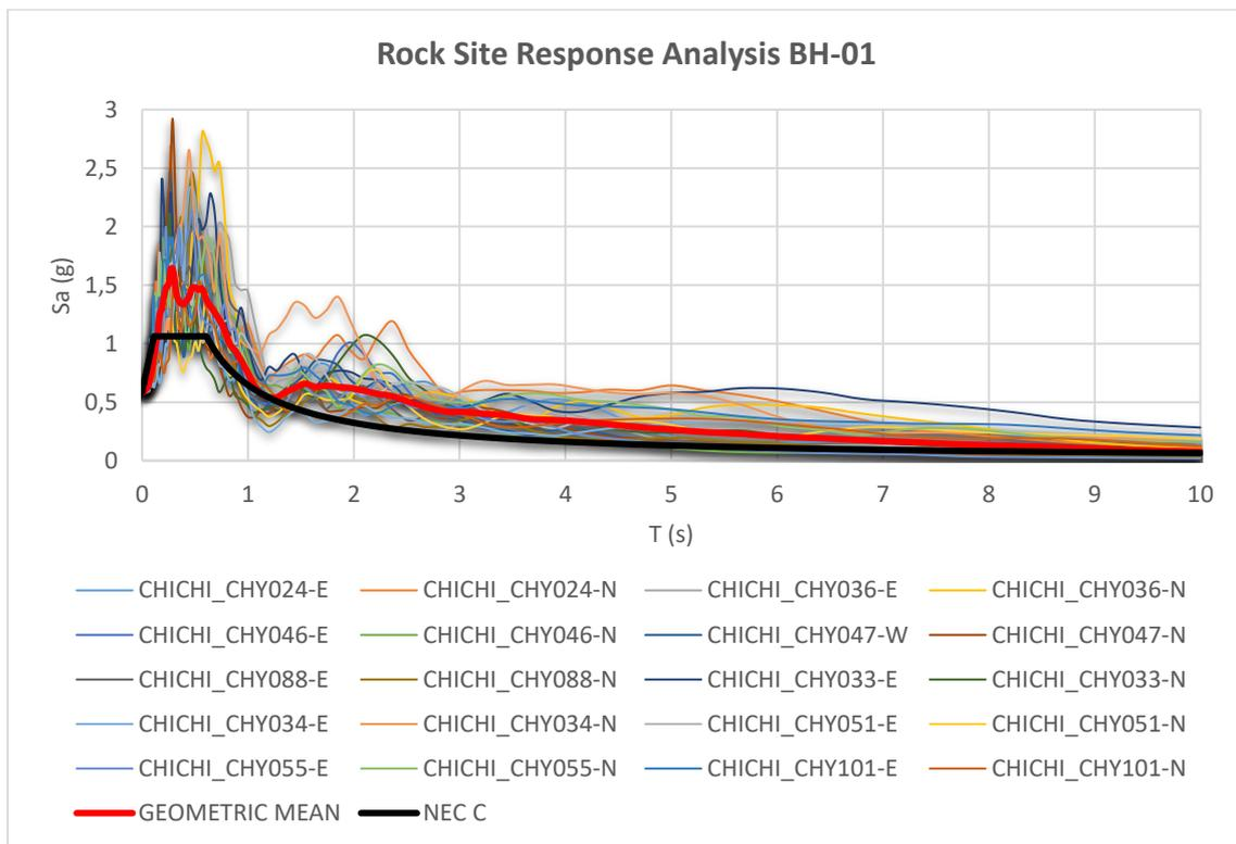
**Figure 12.-** Rock response spectrum for BH-01 and comparison with NEC C spectrum
