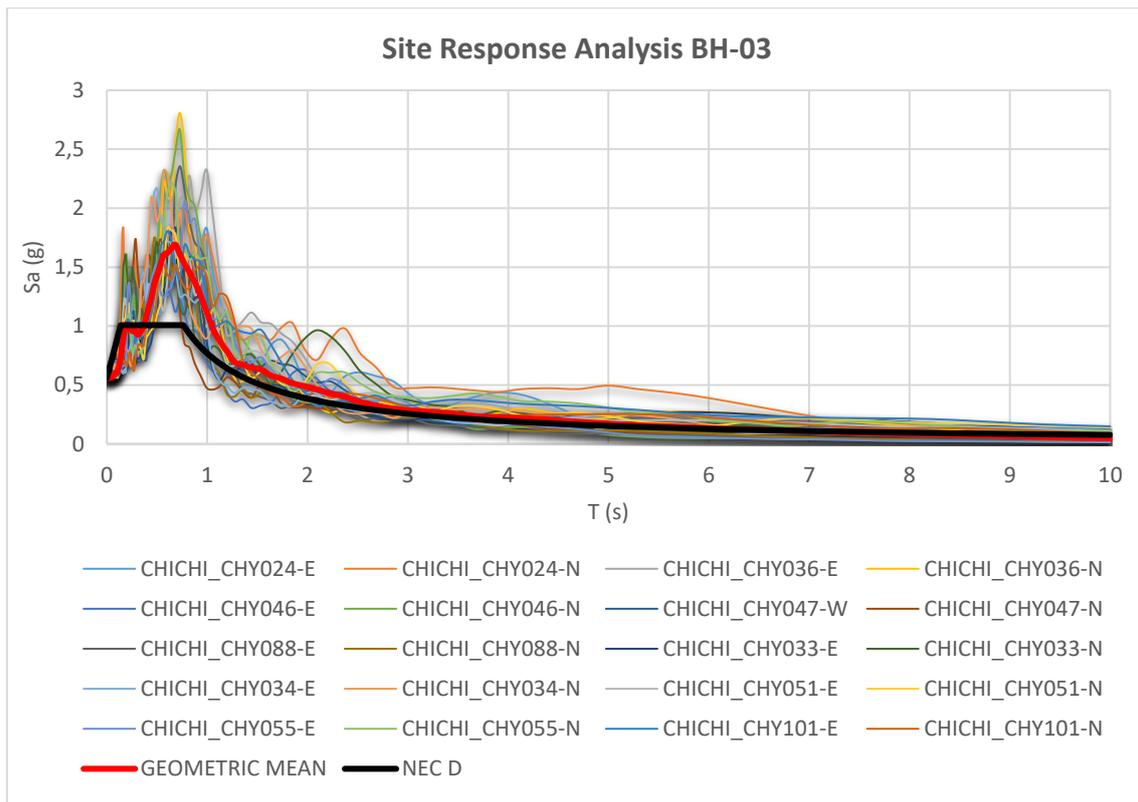
**Figure 8.-** Comparison of acceleration spectra for the 5% structural damping for the horizontal components of the 10 earthquakes for coluvial deposits (ie. BH-03).
