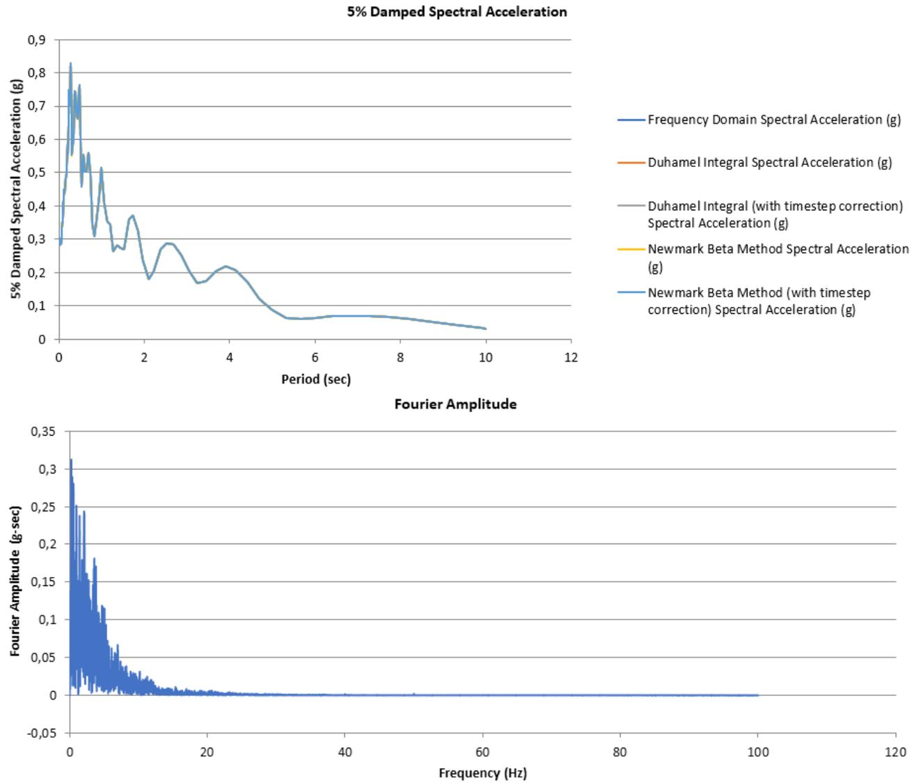
**Figure 7.-** Dynamic parameters of one of the earthquakes considered for the analysis corresponding to 475 years of return period (PEER, Center for the Development of Seismic Engineering of the Pacific).
