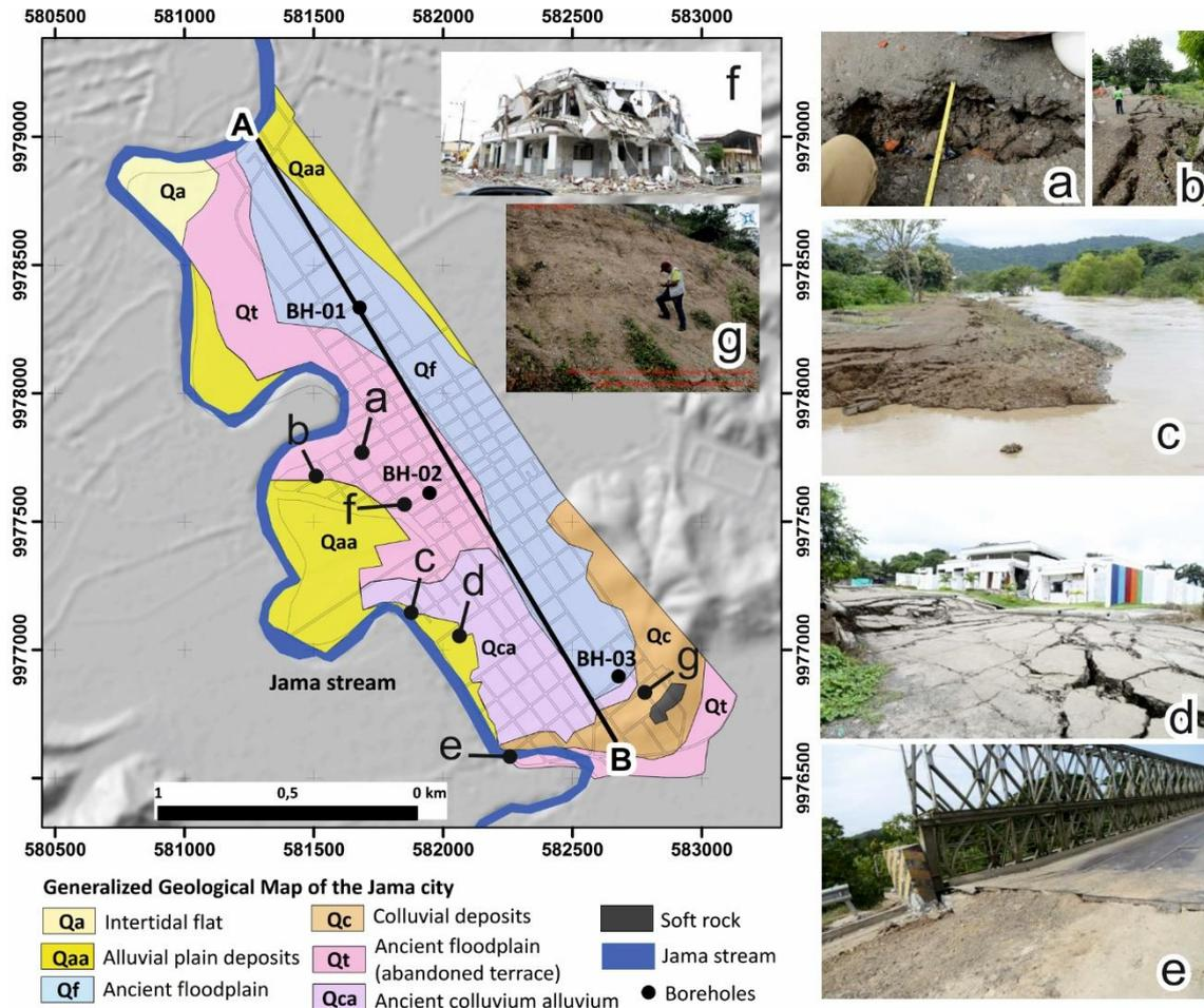
**Figure 3.** Geological map of the urban area of Jama city and earthquake environmental effects documented few days after the M 7.8 2016 earthquake
