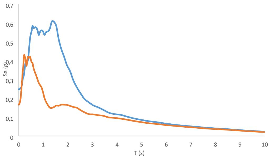
**Figure 10.** Rock and abandoned floodplain strata Surface Response Spectrum for BH-02 sounding. Colors represent: the blue color the surface data and the orange line the rock data.
