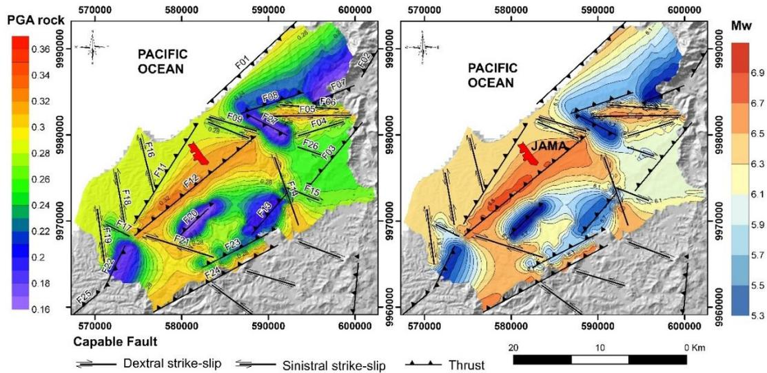
**Figure 2.** Map of maximum magnitudes and PGA-Rock obtained from the analysis of capable geological faults in the Jama canton.
