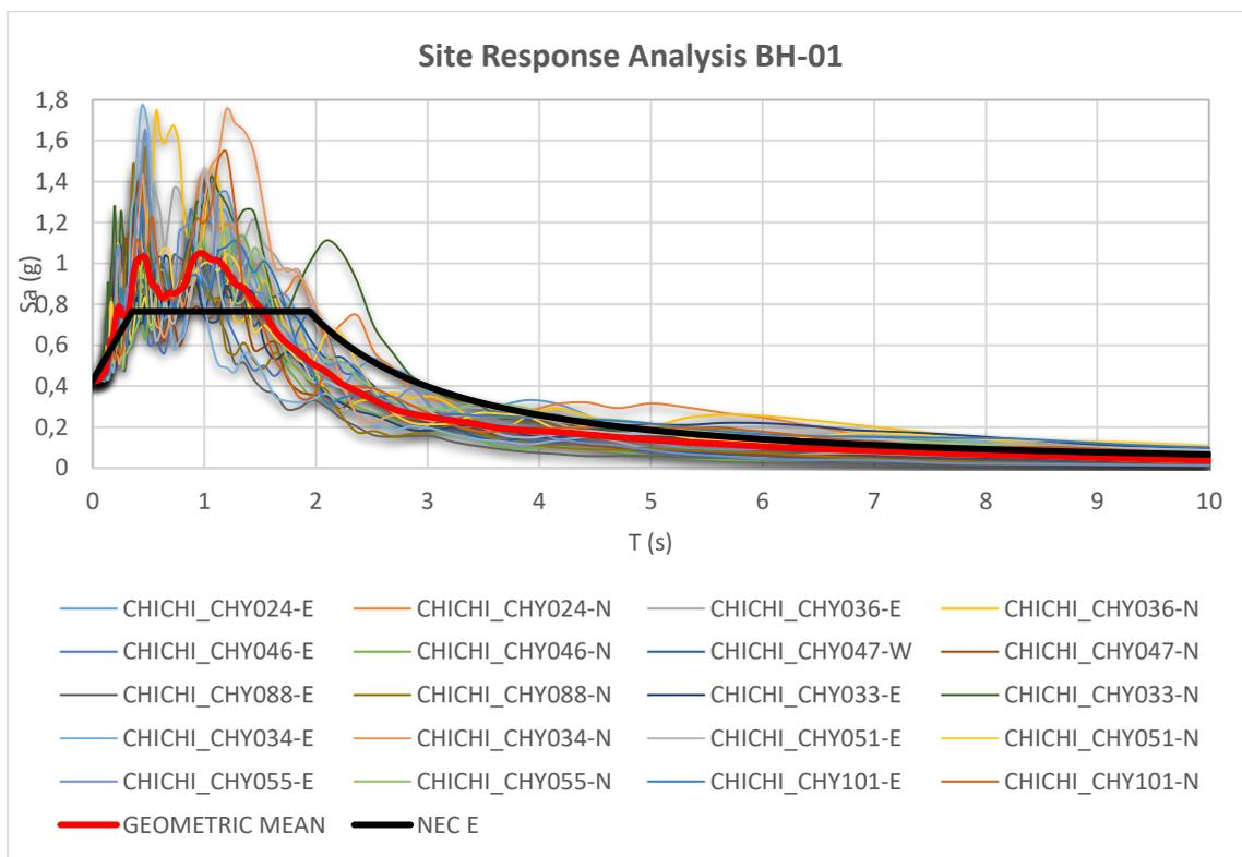
**Figure 9.-** Comparison of acceleration spectra for the 5% structural damping for the horizontal components of the 10 earthquakes for alluvial soils (ie., BH-01).
