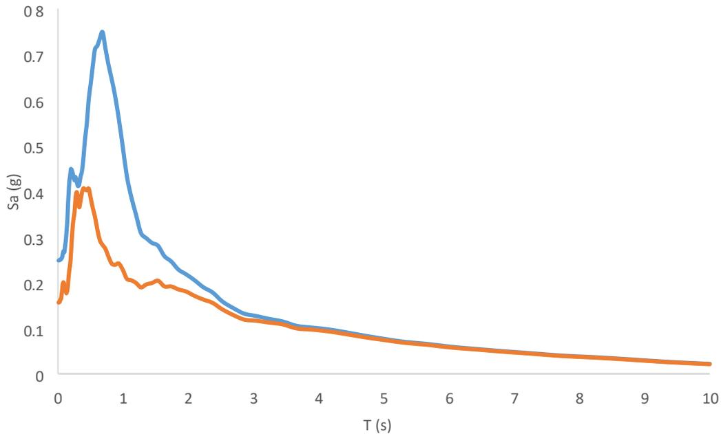
**Figure 8.** Rock and coluvial strata surface response spectrum for the BH-03 well. Colors represent: the blue color the surface data and the orange line the rock data.
