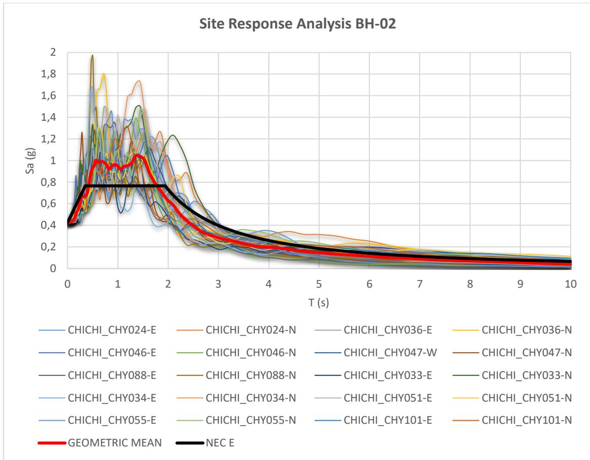
**Figure 10.-** Comparison of acceleration spectra for the 5% structural damping for the horizontal components of the 10 earthquakes for abandoned floplain deposits (ie., BH-02)
