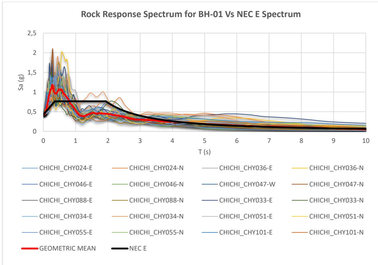
**Figure 15.-** Rock response spectrum for BH-01 and comparison with NEC E spectrum
