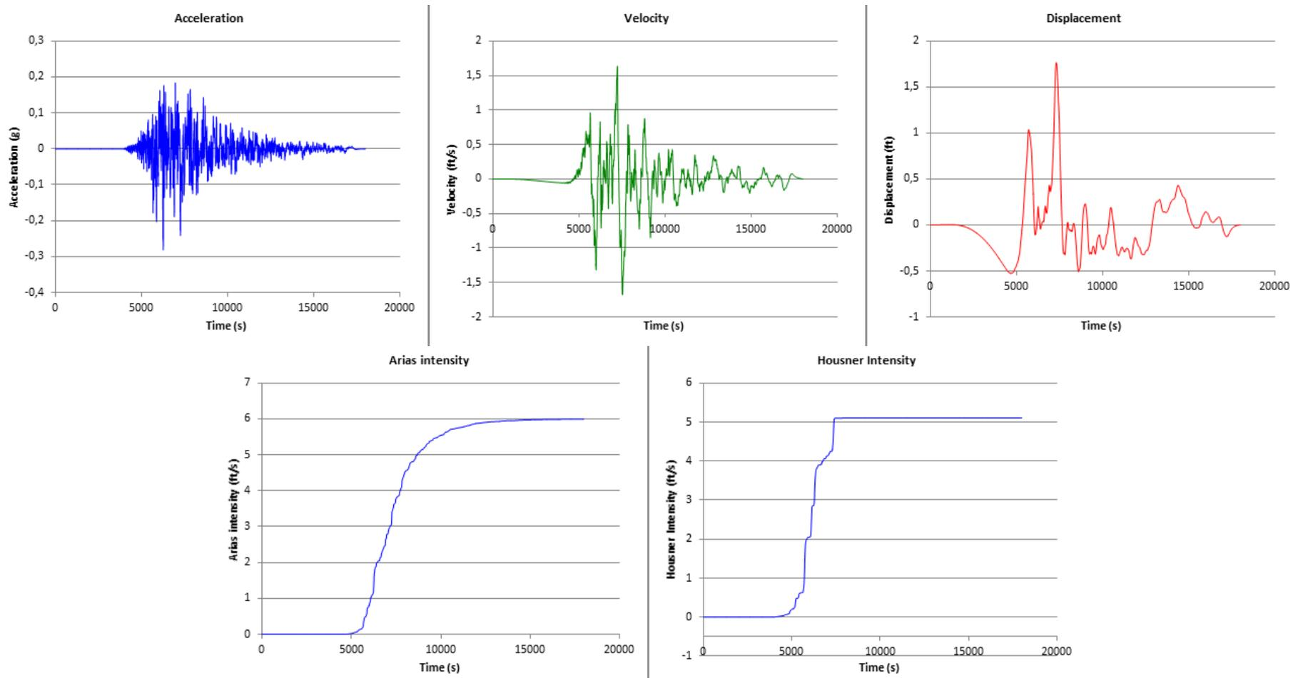
**Figure 6.-** Records time-history and dynamic parameters of one of the earthquakes considered for the analysis corresponding to 475 years of return period (PEER, Center for the Development of Seismic Engineering of the Pacific).
