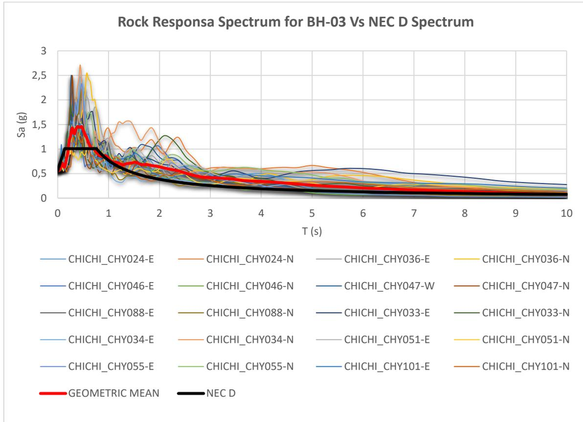
**Figure 14.-** Rock response spectrum for BH-03 and comparison with NEC D spectrum
