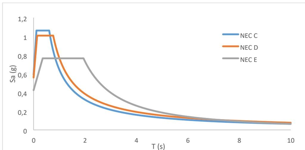
**Figure 6.** Elastic seismic spectra of NEC (2015) accelerations for soil and rock profiles.
