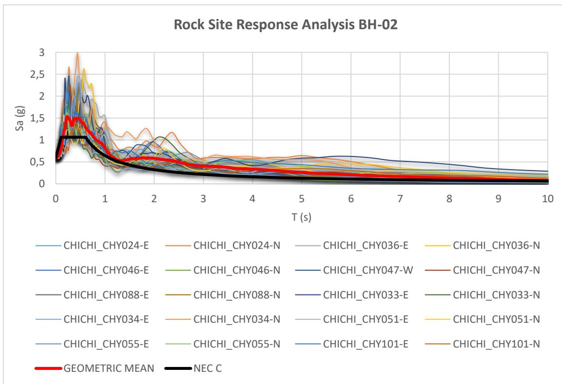
**Figure 13.-** Rock response spectrum for BH-02 and comparison with NEC C spectrum
