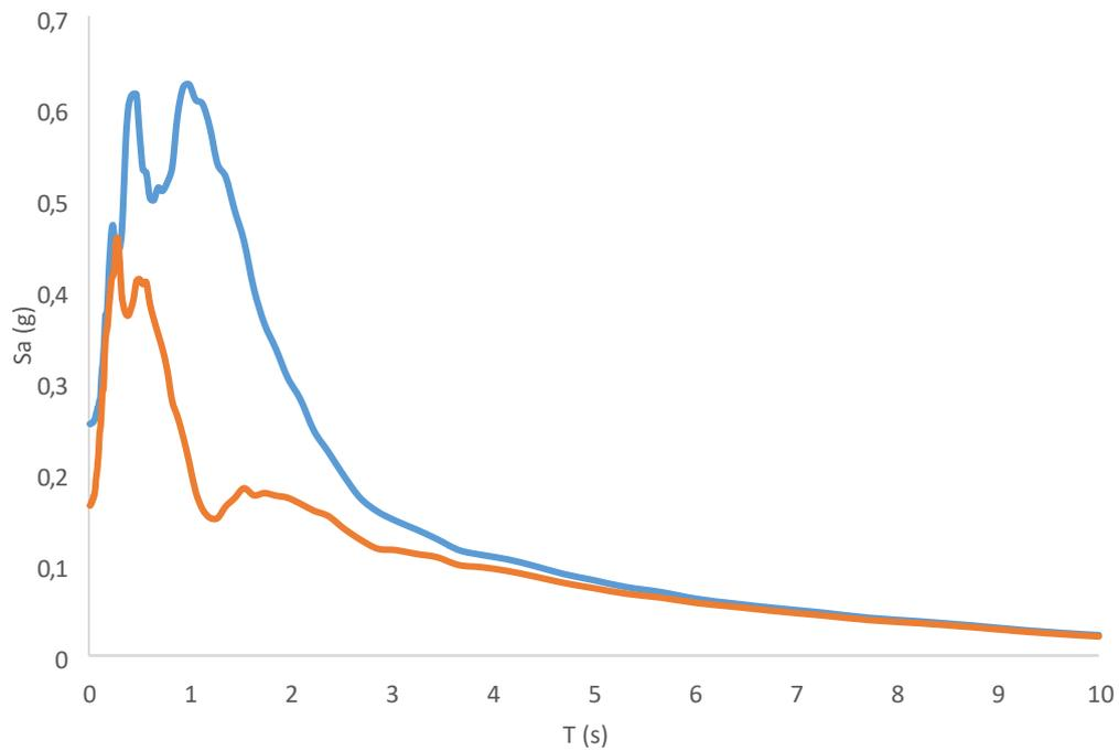
**Figure 9.** Rock and floodplain strata surface response spectrum for the BH-01 borehole. Colors represent: the blue color the surface data and the orange line the rock data.
