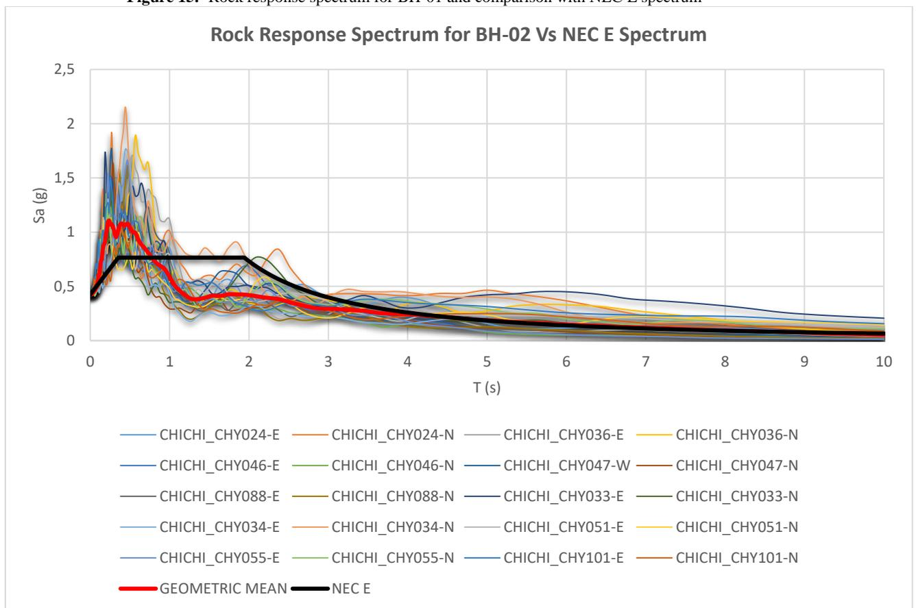
**Figure 16.-** Rock response spectrum for BH-02 and comparison with NEC E spectrum
