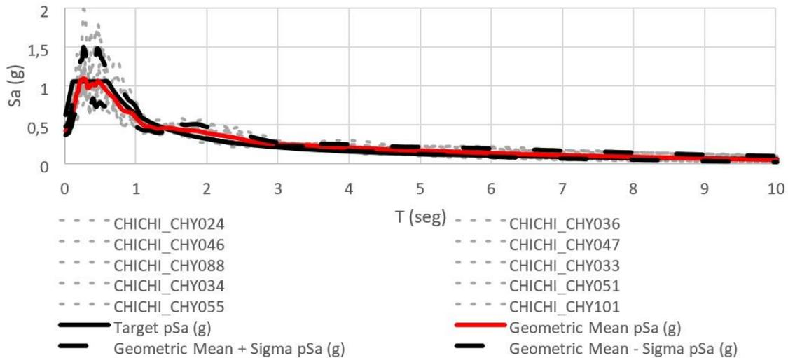
**Figure 7.** Elastic seismic spectra Acceleration response spectrum (5% structural damping) for ten scaled seismic movements (gray lines) for inverse component earthquakes, with seismological characteristics similar to the expected uniform hazard spectrum, 10% probability of exceedance in 50 years, the median and median  $\pm 1$  standard deviation of the scaled movements for NEC-type rock profile.
