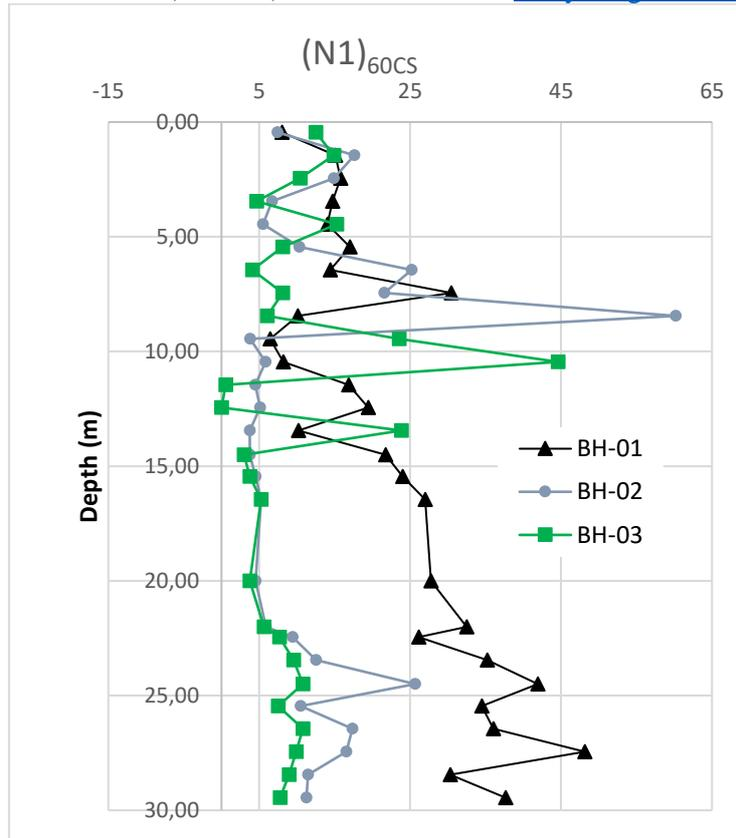
Figure 1.- SPT test results vs depth
