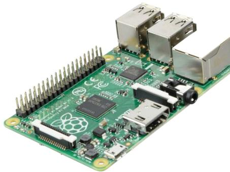
**Figura 3.6 Raspberry Pi 3 modelo B**
