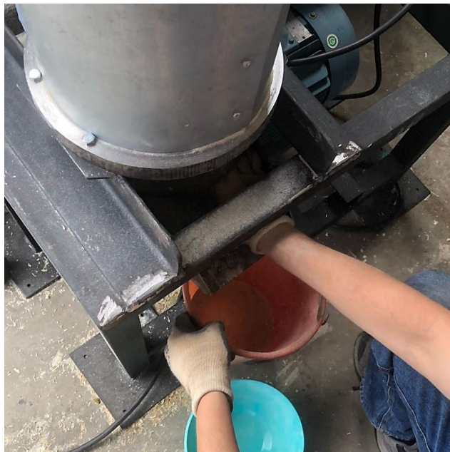
Figura 4.7 Retiro de material residual
