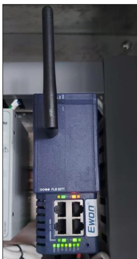
Figura 2.8 Gateway industrial Ewon Flexy 205
