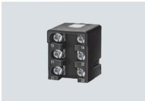
The three-pole contact block with snap-action or slow-action contacts is regularly available for all enclosure forms. The same installation space is required as for a two-pole block. The version with 1 NO + 2 NC offers for example more safety through redundant shutdowns (2 NC contacts) with simultaneous signaling (1 NO contact). The three-pole blocks are also available with make-before-break and with 2 NO + 1 NC.
