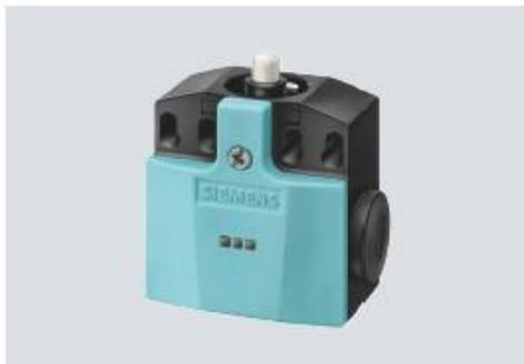
The enclosure versions can be supplied with an LED signaling indicator (1 x green + 1 x yellow). This is the first time that optical signaling equipment is also available for small standard enclosures according to EN 50047. The LED signaling indicators are available in all common voltages (24 V DC and 230 V AC).
