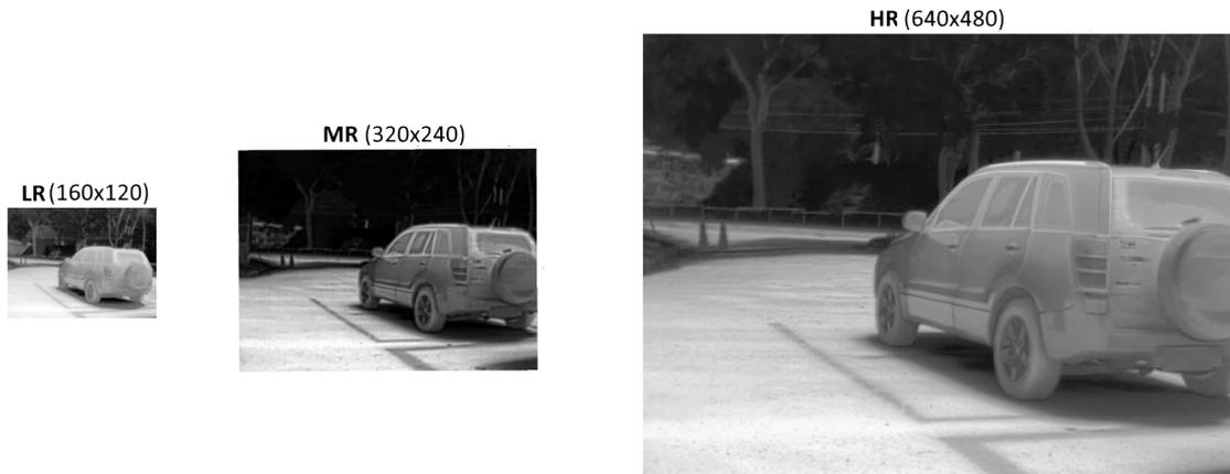
Fig. 3.6 Examples of thermal images acquired by each camera of the second thermal dataset (ThD3-1021). (*left*) LR image with  $160 \times 120$  native resolution from Axis Domo P1290. (*middle*) MR image with  $320 \times 240$  native resolution from Axis Q2901-E. (*right*) HR image with  $640 \times 480$  resolution from FC-6320 FLIR (native resolution  $640 \times 512$ ).
