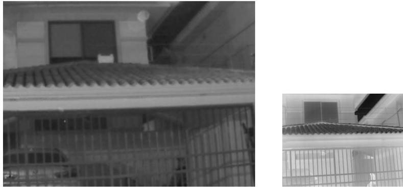
Fig. 1.3 Visible and thermal images of the same scene at night. (*left*) captured with a RGB camera, and (*right*) captured with a thermal camera. Visible image has higher resolution than thermal.
