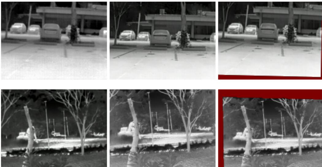
Fig. 3.9 Image registration results. (*top*) From left to right: LR image; MR image; and image resulting from the registration of MR image with the results of  $SR_{LR}$  image. (*bottom*) From left to right: MR image; HR image; and image resulting from the registration of HR image with the results of  $SR_{MR}$  image.
