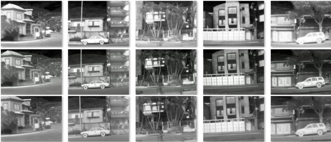
Fig. 3.8 ThD3-1021 dataset examples, thermal images of each camera and their slightly different regions of the scene. (*top – row*) LR images from Axis Domo P1290. (*middle – row*) MR images from Axis Q2901-E. (*bottom – row*) HR images from FC-6320 FLIR.
