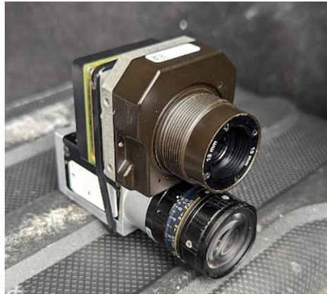
Fig. 3.3 TAU2 (*top*) and Balsar (*bottom*) cameras mounted one over the other.
