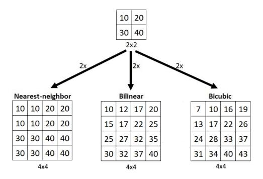
Fig. 2.2 Illustration of traditional interpolation-based methods.
