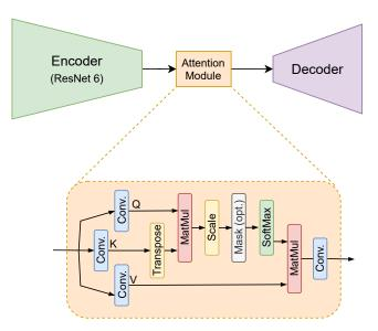
Fig. 4.7 Generator defined by: ResNet-6 as encoder, followed by the scaled dot-product attention module [116] and then the decoder.
