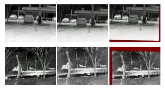
Fig. 3.9 Image registration results. (top) From left to right: LR image; MR image; and image resulting from the registration of MR image with the results of SR<sub>LR</sub> image. (*bottom*) From left to right: MR image; HR image; and image resulting from the registration of HR image with the results of SR<sub>MR</sub> image.
