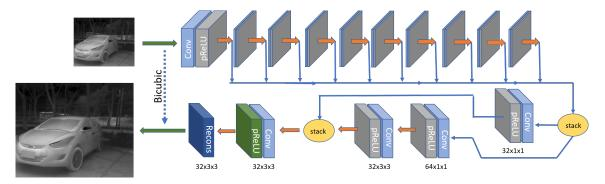
Fig. 4.1 Proposed supervised approach using CNN architecture (TISR-DCNN).
