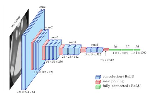
Fig. 2.4 The architecture of the VGG-16 network [105].
