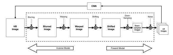
Fig. 2.11 Illustration model employed in most MISR techniques for multi LR generation.
