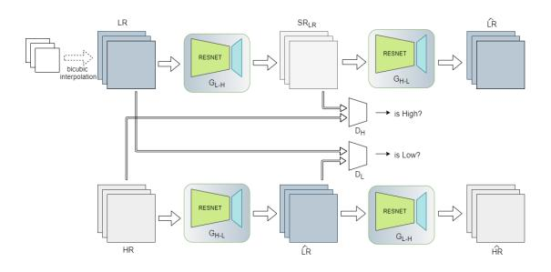
Fig. 4.4 First unsupervised proposed approach (TISR-US-1) illustration, based on a CycleGAN architecture;  $G_{L-H}$  and  $G_{H-L}$  represent generators from lower to higher and from higher to lower resolution, respectively.  $D_H$  and  $D_L$  represent the discriminator for each resolution.
