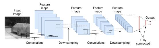
Fig. 2.3 The architecture of a typical convolutional neural network.
