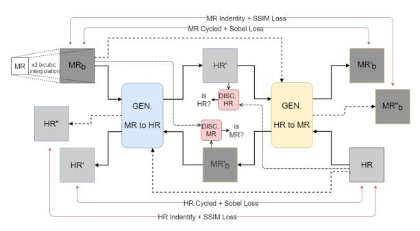
Fig. 4.5 Second unsupervised proposed approach (TISR-US-2) illustration, based on a CycleGAN architecture for MR to HR generator and for HR to MR; with cycled + sobel losses and identity + SSIM losses, and its respective discriminators.
