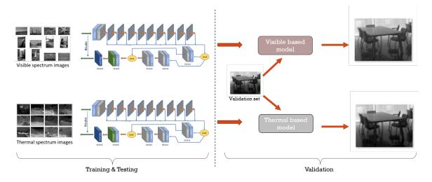
Fig. 4.2 Training process of TISR-DCNN network, which generate two strategies for the testing process.
