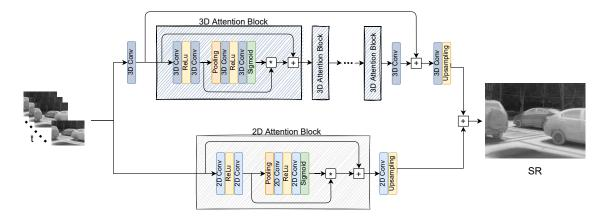
Fig. 5.1 Proposed multi-image thermal super-resolution architecture using a 2D and 3D attention blocks.
