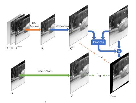
Fig. 2.16 Architecture proposed by NPU-LIFT-LAB [94].
