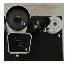
Fig. 3.5 Panel with the cameras for the second dataset: *a*) Axis Domo P1290 (LR); *b*) Axis Q2901-E (MR); *c*) FC-6320 FLIR (HR); *d*) Basler visible spectrum camera, which is not used in the current work.
