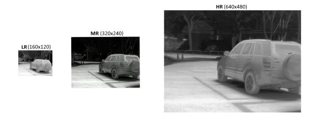
Fig. 3.6 Examples of thermal images acquired by each camera of the second thermal dataset (ThD3-1021). (*left*) LR image with 160×120 native resolution from Axis Domo P1290. (*middle*) MR image with 320×240 native resolution from Axis Q2901-E. (*right*) HR image with 640×480 resolution from FC-6320 FLIR (native resolution 640×512).
