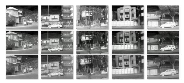
Fig. 3.8 ThD3-1021 dataset examples, thermal images of each camera and their slightly different regions of the scene. (top - row) LR images from Axis Domo P1290. (middle - row) MR images from Axis Q2901-E. (bottom - row) HR images from FC-6320 FLIR.
