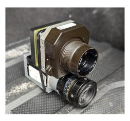
Fig. 3.3 TAU2 (top) and Balser (bottom) cameras mounted one over the other.
