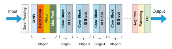
Fig. 2.5 The architecture of the ResNet-50 network [36].
