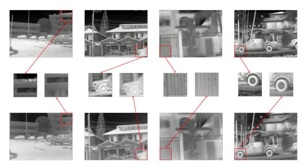
Fig. 4.8 Examples of thermal images acquired in [89]: (top) MR images from Axis Q2901-E (320×240), used in TISR-US-2 and TISR-US-3 approaches as LR images; (*bottom*) HR images from FC-6320 FLIR (640×480) [89]; (*middle*) enlargements to show the miss-registration between the images.
