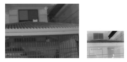
Fig. 1.3 Visible and thermal images of the same scene at night. (*left*) captured with a RGB camera, and (*right*) captured with a thermal camera. Visible image has higher resolution than thermal.
