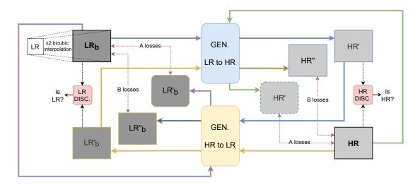
Fig. 4.6 Third unsupervised proposed approach (TISR-US-3) illustration, based on a CycleGAN architecture (for LR to HR and vice versa); *A losses* represents the Sobel and cycled losses, and *B losses* are SSIM and identity losses. Each cycle has its respective discriminators.
