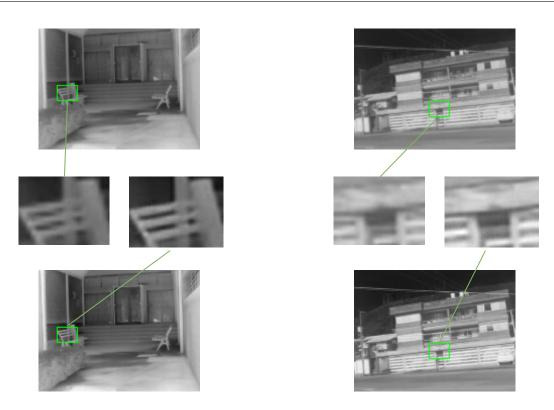
Fig. 5.4 SR results with a  $\times 4$  scale factor: (top - row) results from bicubic interpolation; (bottom - row) results from the proposed approach.
