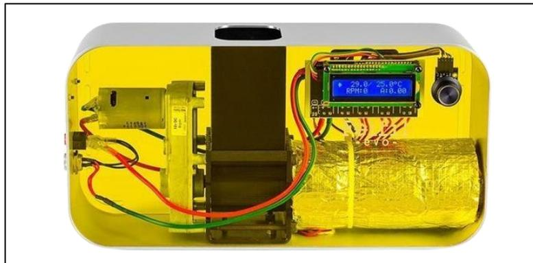
**Figura 1.11 Felfill Evo Filament Extruder [25].**
