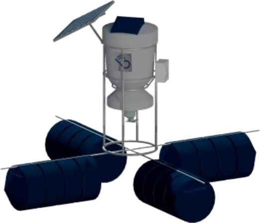
A 3D rendering of a system similar to Alternative 1. It has a hopper with a solar panel on top, supported by a metal frame. This assembly is surrounded by several blue cylindrical floaters. A white control box is also visible on the side of the hopper. |
