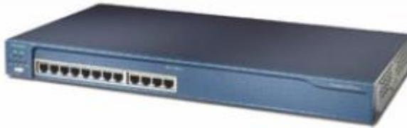
**Figura.4.6.Switch Cisco Catalyst 2950**
