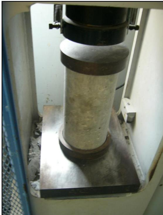
**FOTO 22. ENSAYO A LA COMPRESION**
