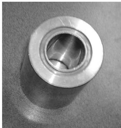
FIGURA 3.3.3 CÁMARA PORTA NÚCLEO #1
